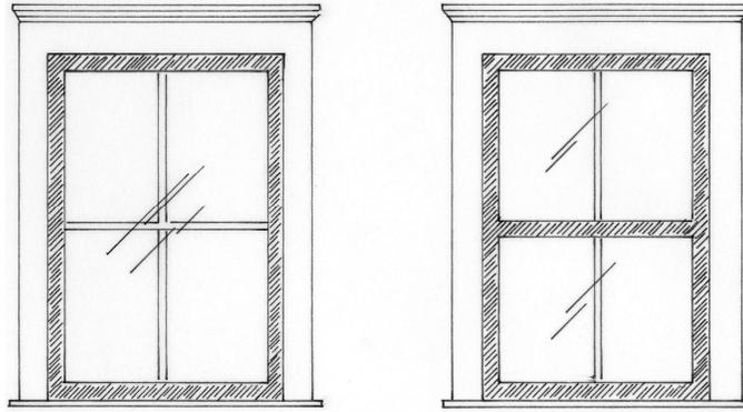
Storm windows should either be full-view or have a center rail in line with the center rail of the window.
